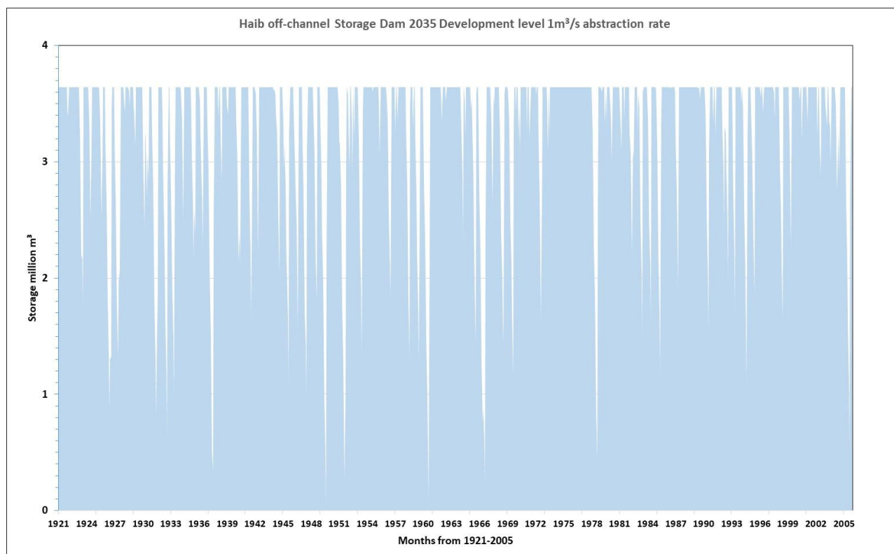
Figure 4-23: Haib off-channel dam storage over the simulation period – Scenario 3g2 1m³/s pumping rate
